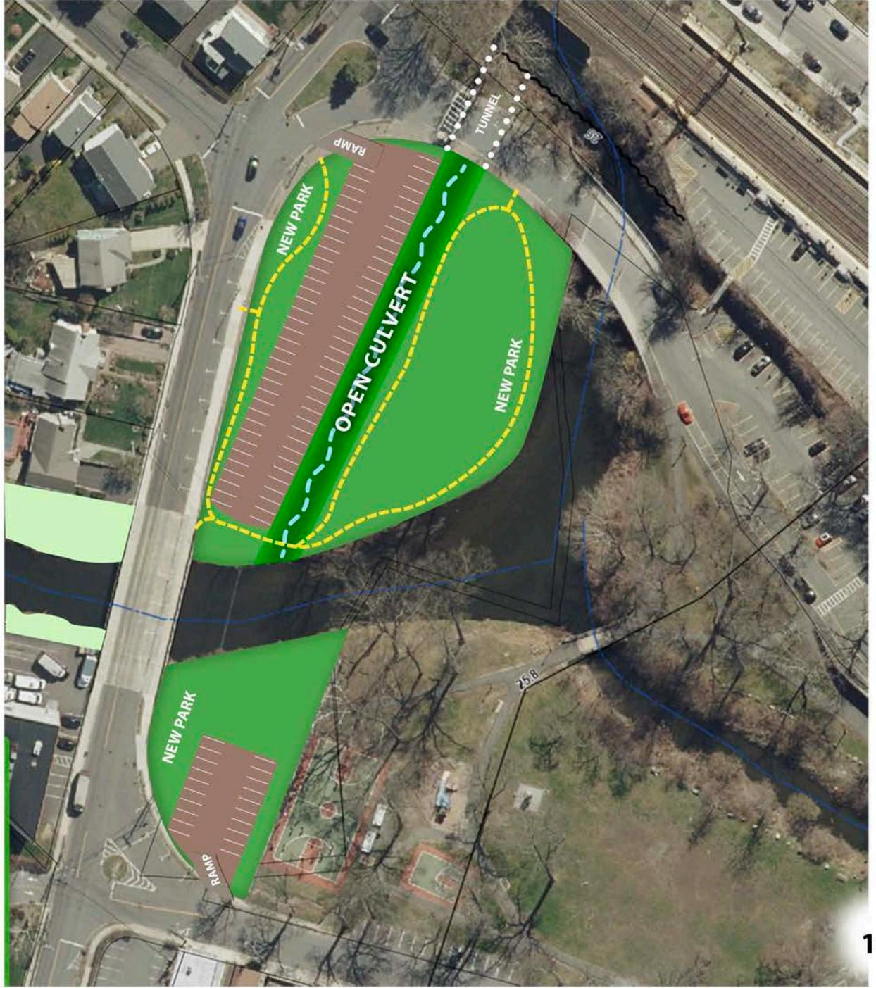
A “tweak” to the Army Corps of Engineers plan for flood mitigation in Mamaroneck converts their proposed tunnel to an open, grass or gravel culvert. The entire area will have pavement removed and be lowered by 3.5 to 5 ft, restoring its floodplain function, improving flood control and allowing for restoration of the park, particularly the river banks. This plan has been endorsed by ACE, the DEC, and the DEC-commissioned SLR study.
