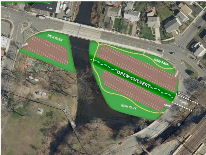
**Open Diversion Culvert & Porous, Floodplain Parking**
