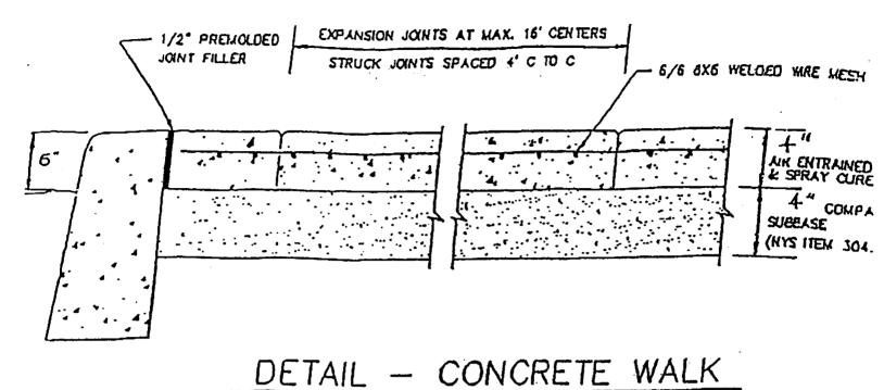
NOTE: PROVIDE 1/2" PREMOLDED JOINT FILLER A.O.B.E.
