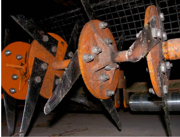
Figure 7-18. Deep slicing can aid with remediating large areas of soil in need of increased infiltration and gas exchange. Source: Frank Rossi.
