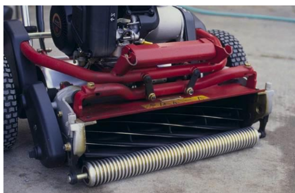
Figure 7-7. Reel mowers are ideal for golf turf mowed under 1" height of cut. Source: Frank Rossi.
