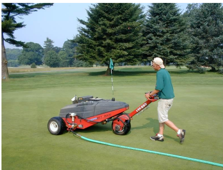
Figure 7-21. Water injection cultivation is the 'gold standard' for increasing infiltration and improved gas exchange with minimal surface disruption. Source: Frank Rossi.
