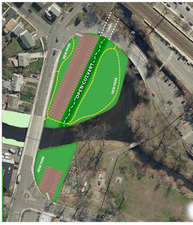
A "tweak" to the Army Corps of Engineers plan for flood mitigation in Mamaroneck converts their proposed tunnel to an open, grass or gravel culvert. The entire area will have pavement removed and be lowered by 3.5 to 5 ft. restoring its floodplain function, improving flood control and allowing for restoration of the park, particularly the river banks. This plan has been endorsed by ACE, the DEC, and the DEC.commissioned SLR study.
