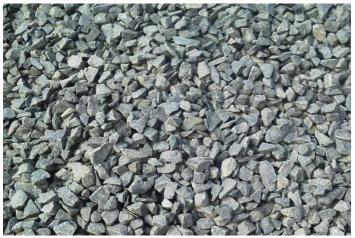
Uniformly sized, highly angular crushed stone
