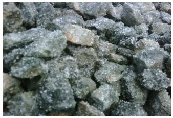
*Close-up of angular stone with Gelscape* **R** *Tackifier applied (prior to admixing with clay loam soil)*
