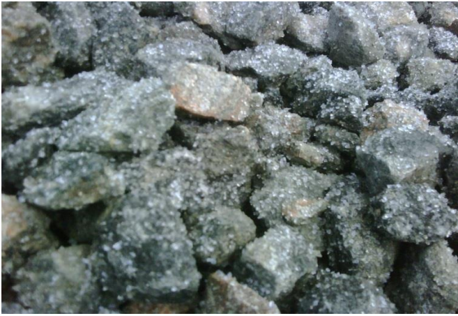
Close-up of angular stone with Gelscape® Tackifier applied (prior to admixing with clay loam soil)
