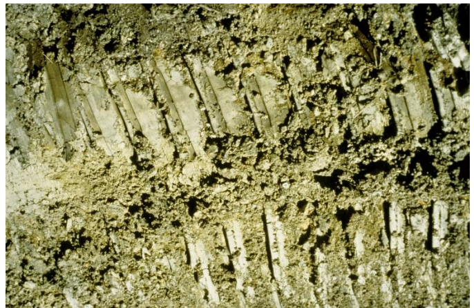
Surface evidence of severe soil compaction
