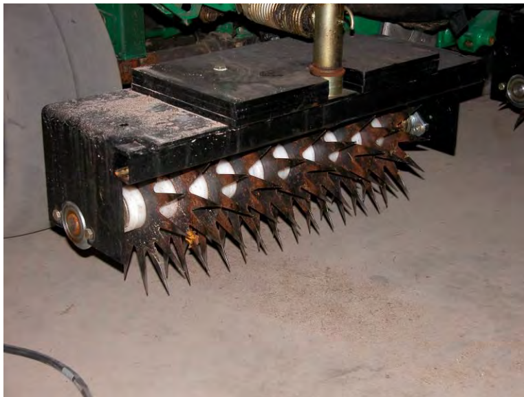
Figure 7-19. Spiking attachments aid with increasing infiltration and can affect significant amounts of surface areas. Source: Frank Rossi.
