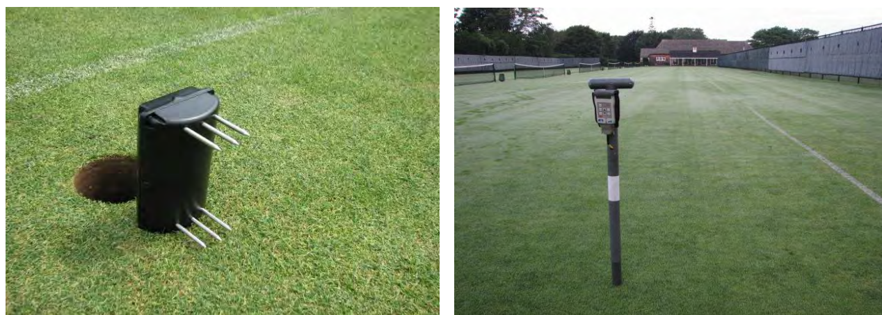
Figure 5-7. Root zone moisture, temperature, and salinity meter (left) and portable moisture meter (right). Source: John J. Genovesi, Maidstone Club
