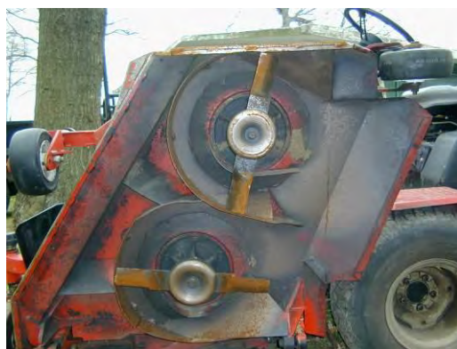
Figure 7-8. Rotary mowers are best used for height of cuts above 1". Blades should be sharpened after every 10 hours of use. Source: Frank Rossi.
