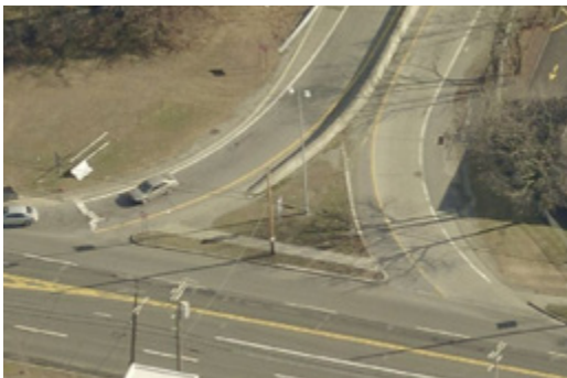
Figure 96: Sidewalks lead to the ramps along Mamaroneck Avenue for entering and exiting I-95, but there are no crosswalks
