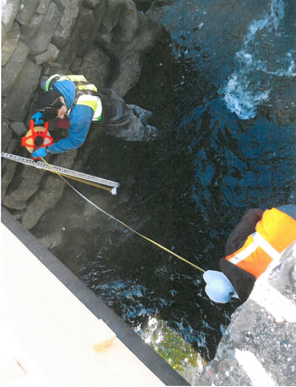
Stream sample BSB-01 and calculating stream cross-section under footbridge.
