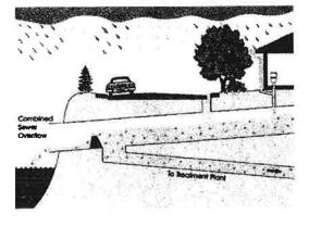
at specific outlets (right) and discharge untreated wastewater directly to nearby streams, rivers or lakes, in order to avoid backups into basements or onto streets. This is a *combined sewer overflow*, or *CSO* for short.
