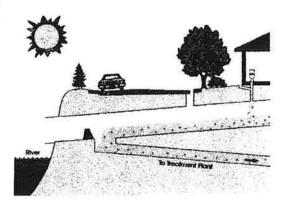
Many of New York State's older cities use combined sewer systems — sewer systems that collect stormwater runoff, domestic sewage and industrial wastewater in the same pipe. Most of the time, combined sewer systems transport all of their wastewater to a sewage treatment plant, where it is treated to
