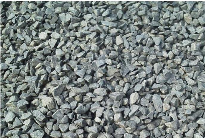
*Uniformly sized, highly angular crushed stone*
